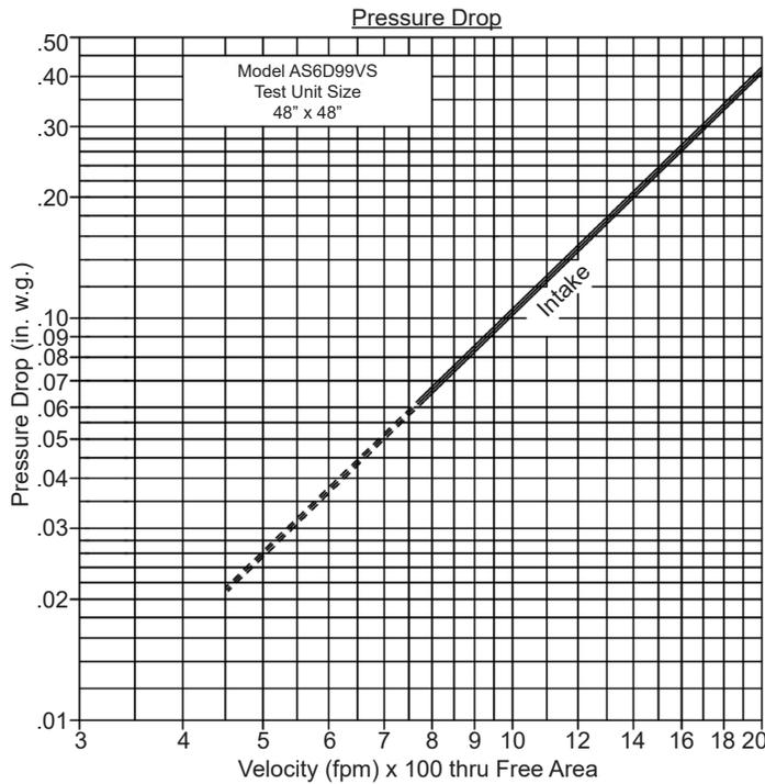
Intake air converted to standard air density.
